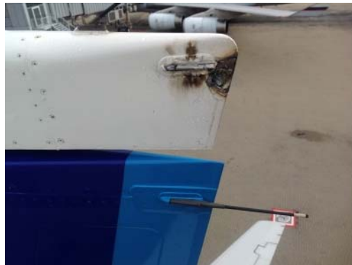
Fig1.2 翼端部への被雷
